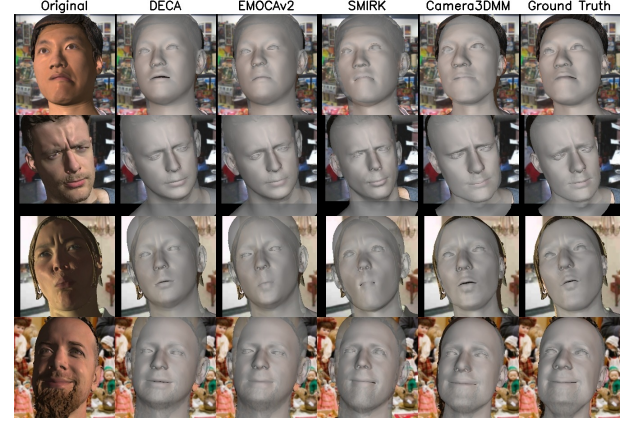
Figure 5: FLAME meshes predicted by DECA, EMOCaV2, SMIRK, and Camera3DMM(Ours) against ground truth.
