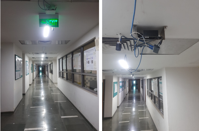
Fig. 6. View of the Testbed with Cameras and Jetson Nanos mounted on the ceiling
